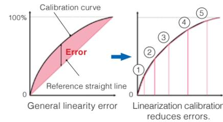
By linearly interpolating between any five points, an output with little error close to the output characteristics can be obtained.
