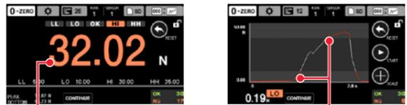
Continuous judgment is conducted when "CONTINUE" is the status displayed on the screen. Support for 4 contacts of high high limit, high limit, low limit, and low low limit. OK/NG judgment in real time for the load value for a certain value.
