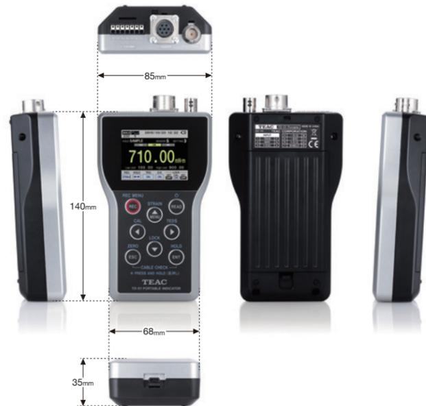
W85 mm x H140 mm x D35 mm (without protrusions)
